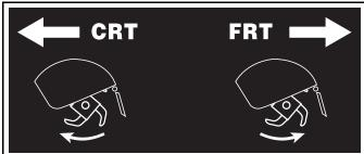
The tine direction selector (found in the lower left area the handle panel) is used to alternate tine rotation between FRT mode (Forward Rotating Tines) to CRT mode (Counter Rotating Tines).
